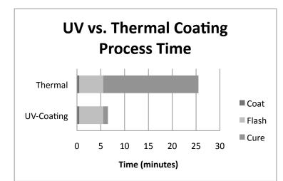
Figure 1. Comparison of general processing times for UV and thermal cure coatings
